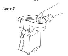
2. Place the juice collector / bowl onto the top of the motor base.
